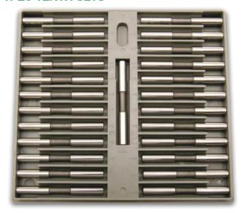
Consists of a center Nominal Gage, plus 12 gages in .0001" STEPS RANGING DOWNWARD from the nominal and 12 gages in .0001" STEPS RANGING UPWARD from the nominal.
